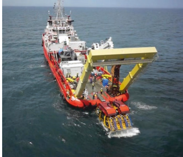
Fig. 27 Sea trial of a pilot mining robot (MineRo II)
