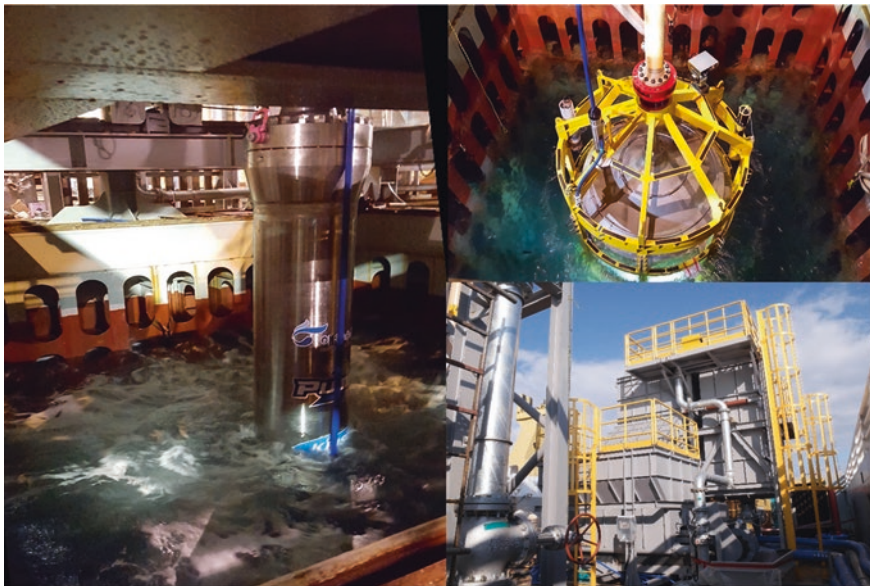
Fig. 32 Photos at sea trial of lifting system: lifting pump launching, buffer station, and on-board separation and measurement facility (from left clockwise)
