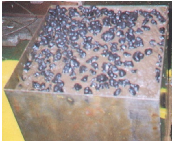
Fig. 13 Partially buried nodules on top of box core
