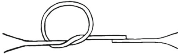
Fig. 7.4 Schematic of a microfiber knot resonator using a second microfiber as collecting fiber [8]
