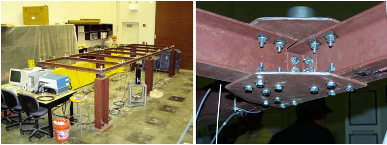
Fig. 26.1 Laboratory setup of the UCF Grid (left) and beam to girder connections (right) [15]
