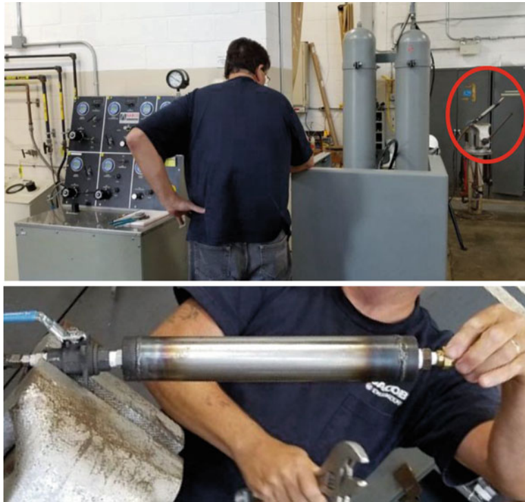
Fig. 4.5 In the top image, complete hydrostatic proof test set-up with pressure gauges to the left and the designed pressure vessel clamped in the background on the right, circled in red. In the bottom image, a close view of the pressure vessel being vented initially during the hydrostatic proof test as the vessel fills with water at a low pressure
