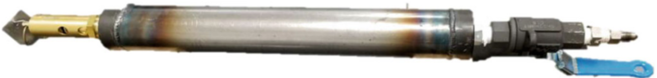
Fig. 4.1 Final manufactured pressure vessel with pressure system components attached. The fill valve and K-bottle connection are shown on the right, the pressure vessel centered, and the relief valve to the left
