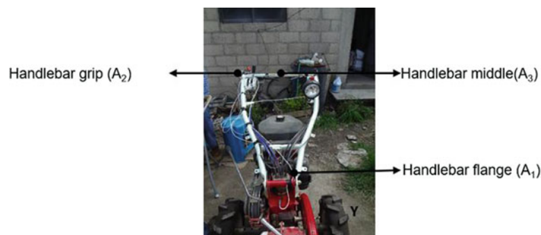
Fig. 36.4 Location of accelerometers on the handlebar structure
