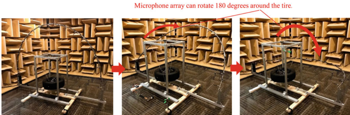
Fig. 34.1 Experimental set-up inside Virginia Tech anechoic chamber
