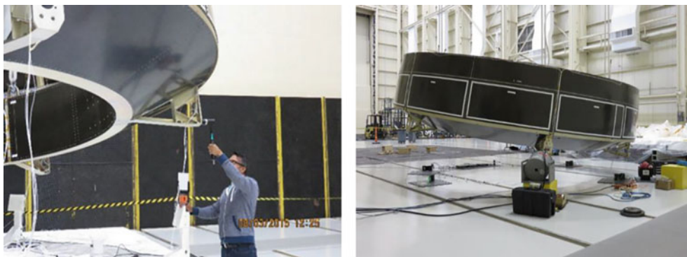
Fig. 25.6 CMA simulator test setups: impact hammer (left)—multi-shaker setup (right)
