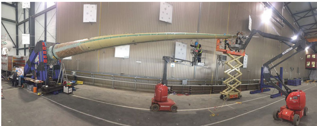
Fig. 10.9 Setup of measurement campaign on wind turbine blade
