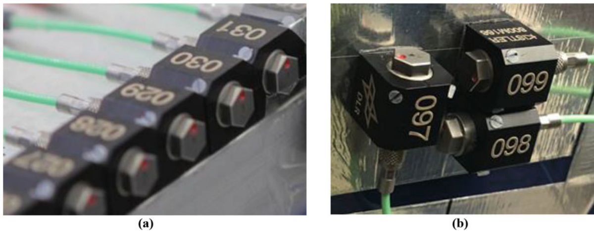
Fig. 10.8 Sensor installation. (a) uni-axial application. (b) tri-axial application
