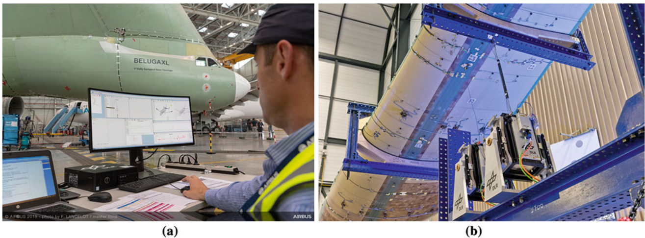
Fig. 10.2 Recent ground vibration tests performed by the German Aerospace Center from Göttingen Germany. (a) Beluga XL ground vibration test in June 2018 [11]. (b) Wind turbine blade modal testing in Feb. 2018
