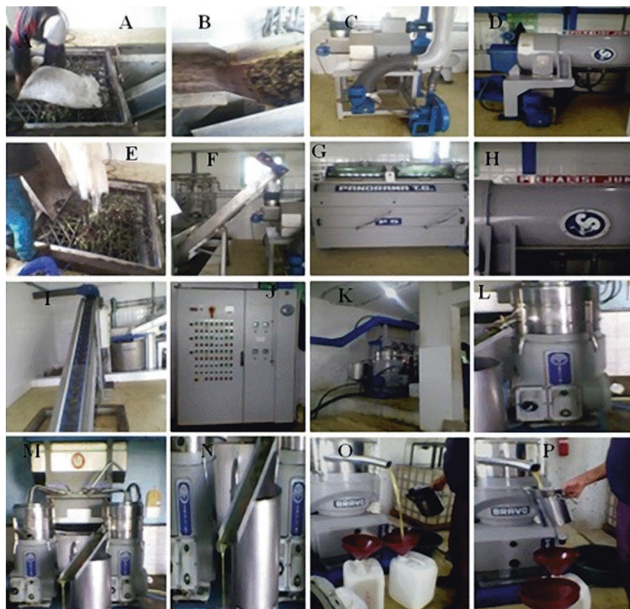
Picture 4.3 Steps of olive oil production by continuous extraction system. (a, b, e, i) triage, selection, leaf removing and washing; (c, d, g, h) decanter and separation of phases; (k–p) clarification of olive oil. (Photos taken by authors)
