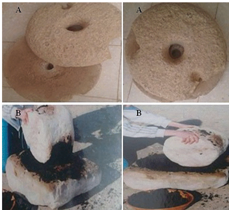
Picture 4.1 The artisanal processes of crushing olive fruit to produce olive oil in Tunisia. (Photos by Issaoui M). (a) (Top row, left and right): Granite stone wheels that rotate around an axis to grind the olives. (b) (Bottom row, left and right): Manual artisanal method for crushing full ripe olives to obtain olive oil. The paste is repeatedly pressed between stones, while oil drains into a container, held at a lower level. (Photos by Issaoui M. and taken in Tunisia; Issaoui et al. 2009)
