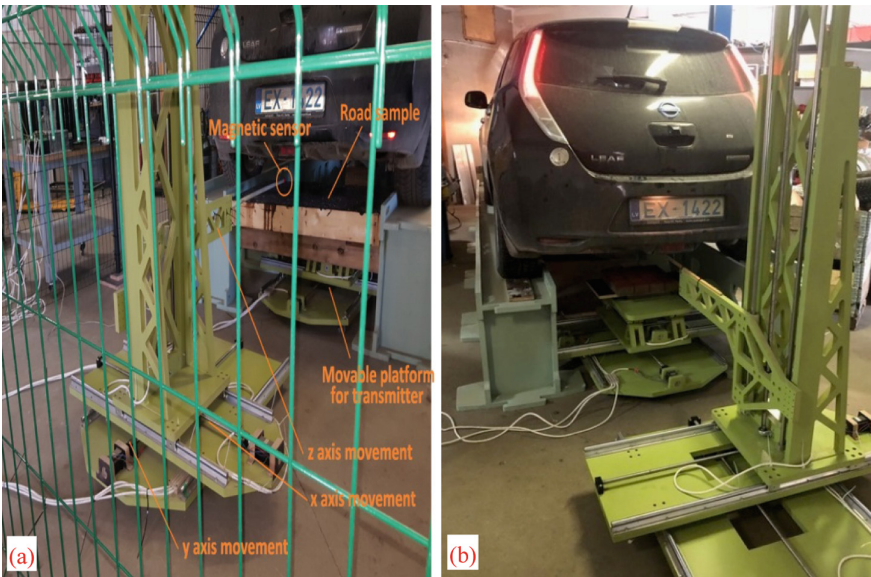
Fig. 3. The test bench for the research influence of constructive materials of road cover on magnetic field dispersion: a—general view; b—the platform under an electric vehicle.
