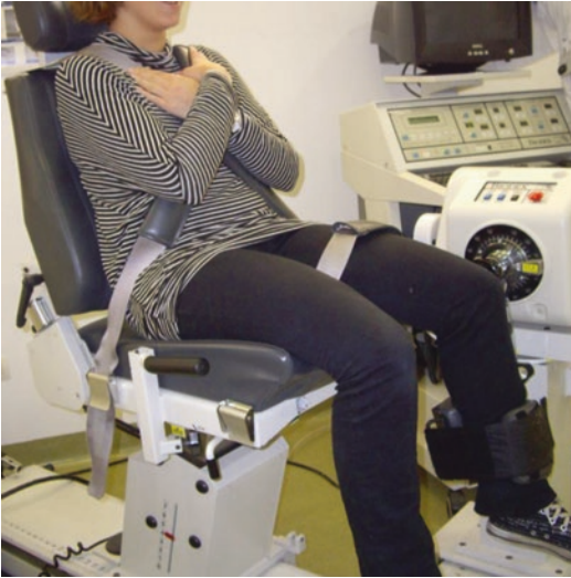
Fig. 7.2 Isokinetic dynamometry machine. The maximum moment of force as well as the agonist-antagonist torque ratio can be accurately evaluated. It also allows treatment at constant speed, both in concentric and eccentric mode
