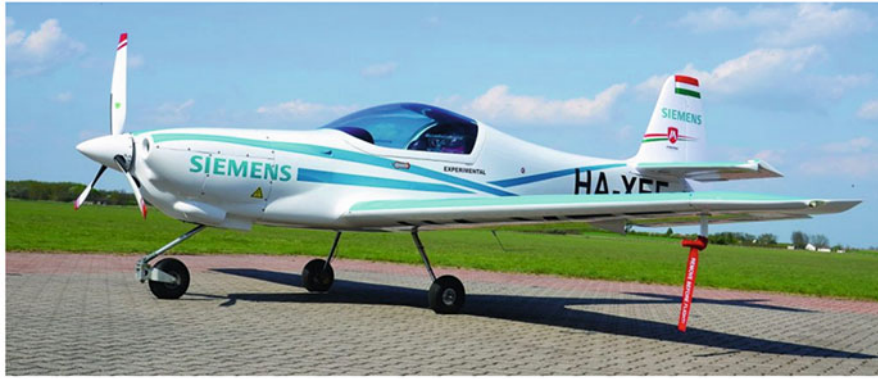
Fig. 6.4 The eFusion battery operated small aircraft
