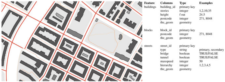
Fig. 1 Initial objects represented in the proposed data model: buildings, blocks, and streets. Source Cadastral survey of Canton Zurich and ©2011 Swisstopo (JA100120)
