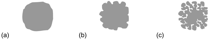
Fig. 2 Convolution. The perimeter increases relative to area, from the most compact (a) to least compact shape (c)
