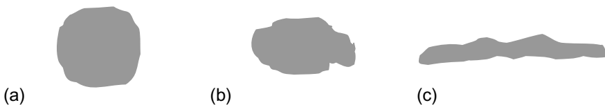
Fig. 1 Elongation. The diameter increases relative to area, from the most compact (a) to least compact shape (c)
