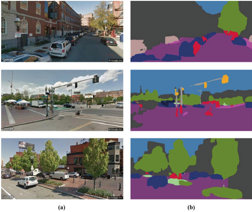
Fig. 8 Image classification results on GSV images using pyramid scene parsing convolutional neural network
