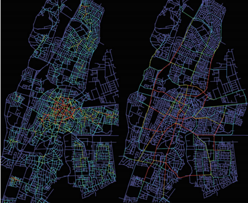
Fig. 9 Angular choice analyses with a low (left) and high (right) metrical radius for Haarlem
