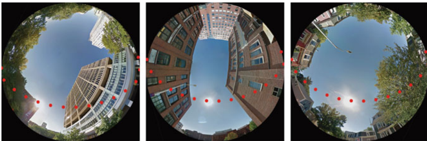
Fig. 5 The overlay of the sun path of September 1st, 2014 on three hemispherical images taken in September
