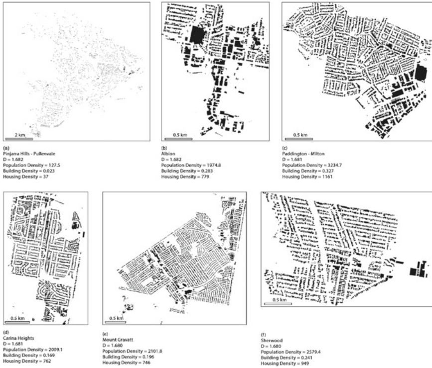
Fig. 7 Examples of selected neighbourhoods with similar fractal dimensions. The building footprints data were extracted from Google Maps
