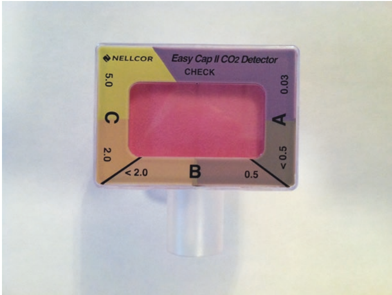
Fig. 1.5 Nellcor Easy Cap II qualitative, colorimetric CO 2 detection device. The purple pH-sensitive paper in the center will change to a yellow/gold color as indicated on the perimeter of the device as increasing levels of CO 2 are detected
