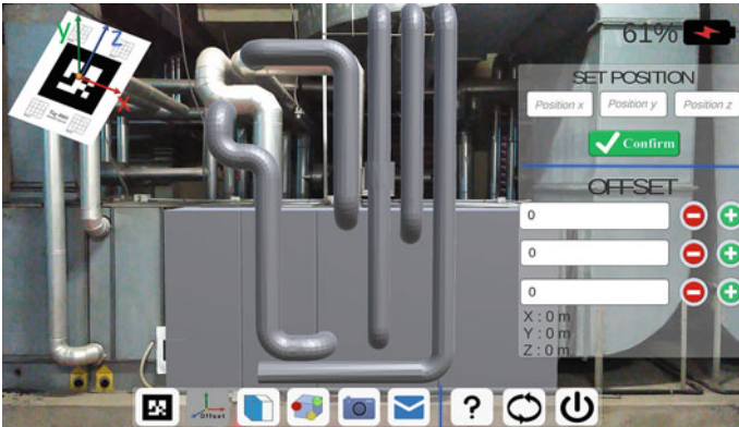
Fig. 3. 3D model augmented on the AHU and menu for fine positioning operations
