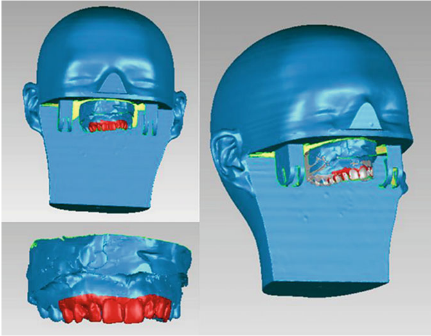
Fig. 8. The digital reference model obtained by the alignment of the digital maxillary model (down to the left) to the digital dum's model (up to the left). In red the surfaces selected for local alignment
