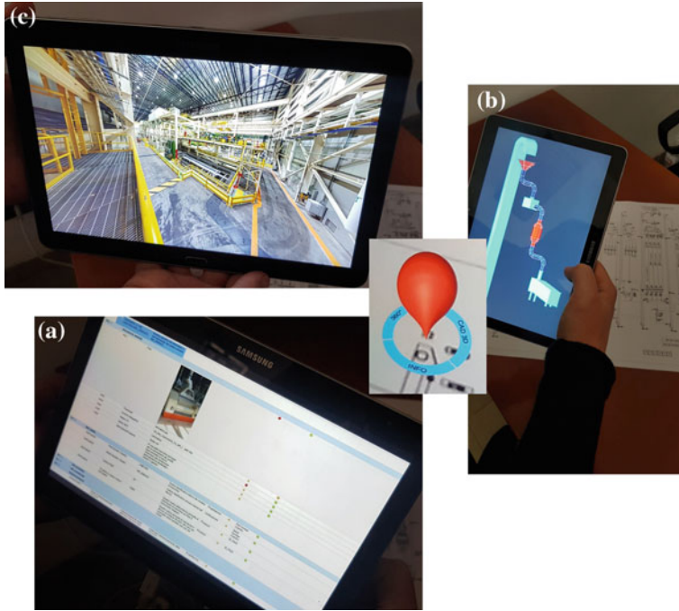
Fig. 5. Visualization of additional technical information through a pie menu: a technical chart with information retrieved from a database (a), a navigable 3D CAD model (b), and a 360° image of a plant section (c)
