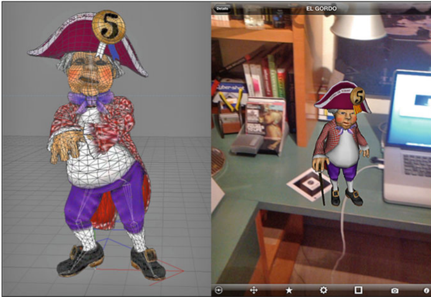
Fig. 5. Version with articulated bones of the model used for animation. On the right display of the model in augmented reality through a mobile device
