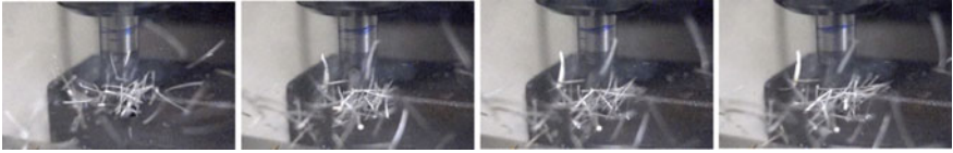
Fig. 5. Sequence of four consecutive video frames, milling with the optimized tool
