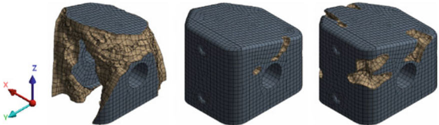
Fig. 9. The final shape of the optimized object for the 35% of infill density for Dep_{xy} (left), Dep_{yz} (middle) and Dep_{xz} (right)
