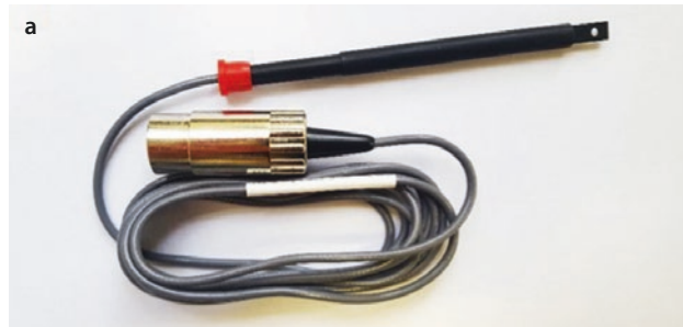
■ Fig. 16.6 Force transducer. a Force transducer. b Schematic of strain gauge circuit
