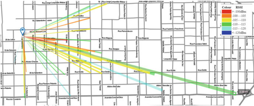
Fig. 11.4 A view of TTN mapper application of the gateway described above. A 2.39 km coverage can be observed in the gateways built by the authors in the city of Ijuí, in the state of Rio Grande do Sul, Brazil
