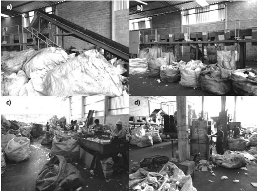
Fig. 6.1 CORESO cooperative. (a) Mechanical treadmill transporting material for initial triage. (b) Initial triage, sorting out, for instance, metal from plastic. (c) Sorting out different types of plastic. (d) Compaction, reducing transportation requirements
