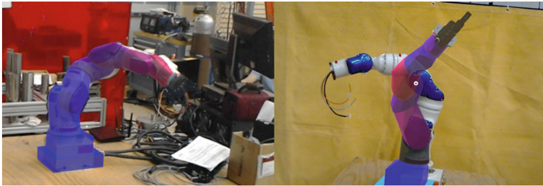
Fig. 2.4 A screenshot of the Hololens application in action. Left : The physical robotic arm has just moved to the position of the holographic arm. Notice the overlay of the hologram onto the physical robotic arm. Right : The hologram “Preview Motion Plan” operation, providing torque feedback via color media
