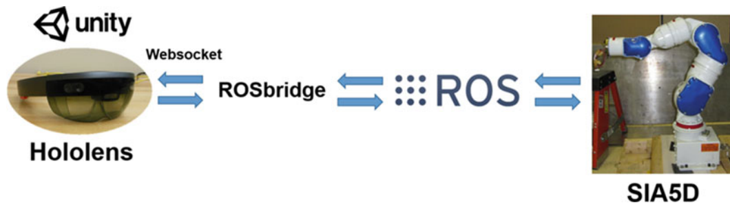
Fig. 2.1 The transmitting/reception layout connecting the Hololens to the SIA5D robot
