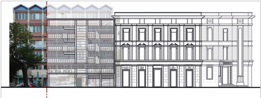
Fig. 4. Survey and comparison between the building and the A. De Cecco project
