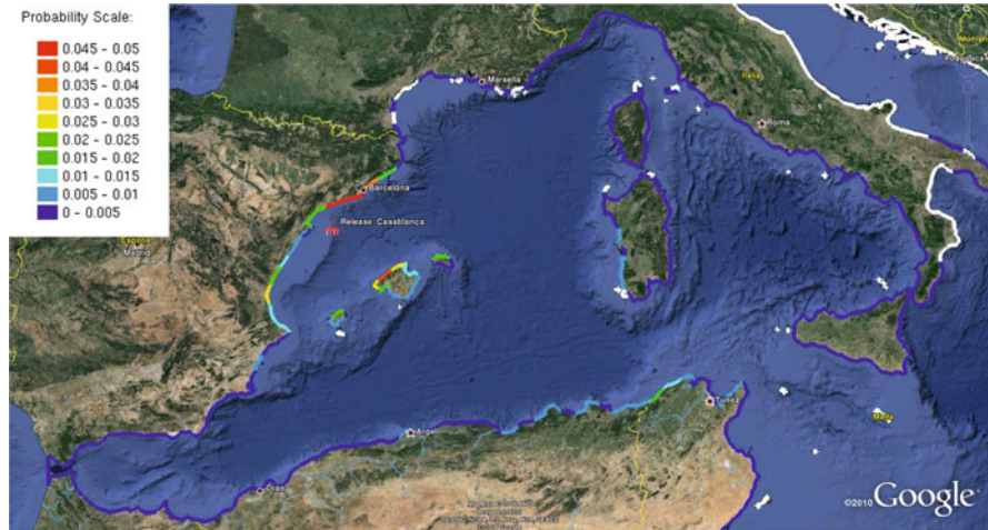
Fig. 6 Beaching probability map for a spill produced at the Casablanca oil platform (the red platform icon in the image). The vertical line in Gibraltar Strait indicates the percentage of particles which reach the Atlantic Ocean
