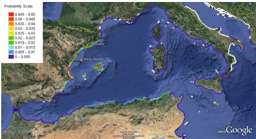
Fig. 4 Beaching probability map for a spill produced at Woodford sunk position (the vessel icon in the image). The vertical line in Gibraltar Strait indicates the percentage of particles which reach the Atlantic Ocean
