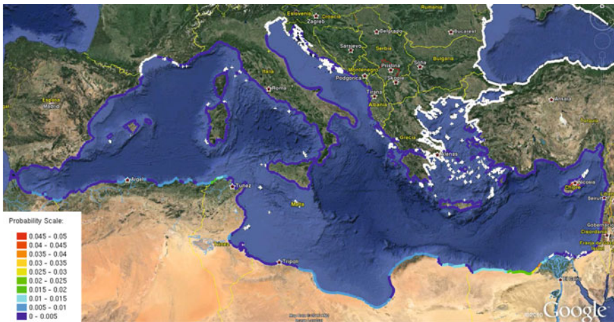
Fig. 9 Oil beaching probability map associated with the main oil tanker route joining the Suez Canal with the Gibraltar Strait. The vertical line in Gibraltar Strait indicates the percentage of particles which reach the Atlantic Ocean
