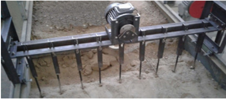
Fig. 8. Industrial platform with feed elements (1 row), installed in the trough of the vibroscreen on the basis of data analysis of finite element modeling.
