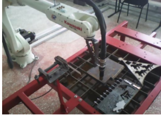
Fig. 1. The robot's arm equipped by UPR device for plasma cutting of metals
