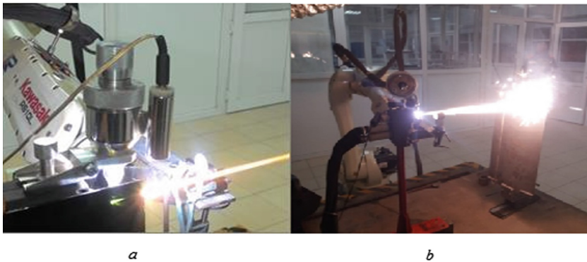
Fig. 2. Robotic processes of microplasma spraying of powder (a) or wire (b)
