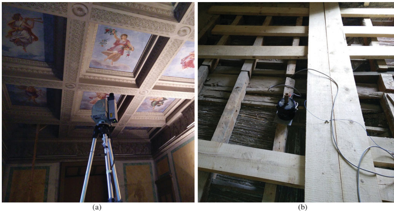
Fig. 1.4 Test setup. (a) LDV during measurements. (b) Shaker position during measurements
