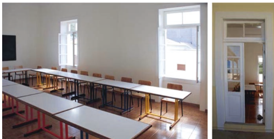
Fig. 3.74 Interior of a school in Mindelo. (1) The inner openings have a generous height, allowing the flow of ventilation at a higher level and contributing to a good performance in terms of natural lighting. (2) Open windows for natural ventilation when the outside temperature is comfortable during the day
