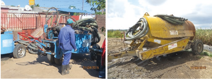
Fig. 16.11 Vacutug (on the left) and vacuum trucks (on the right) operating in Maputo, Mozambique
