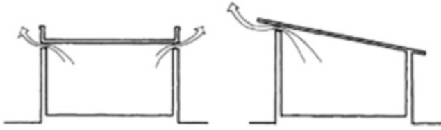
Fig. 3.95 In the case of pitched roofs, the opening should be in the higher wall
