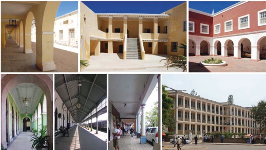
Fig. 3.41 Fixed shading: Arcades. (Above) island of Mozambique (XVIc.), (below) Maputo, Mozambique
