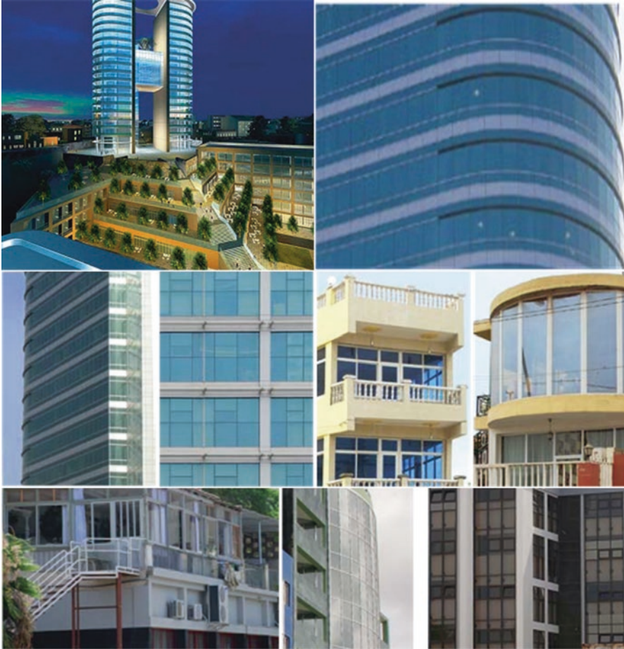
Fig. 3.61 Large glazing areas should be avoided in the facades' typologies, as they are largely responsible for the overheating of the building and subsequent use of energivorous air conditioning systems. The sealed facades with large areas of glazing are an imported typology, inadequate to the hot climates (Luanda, Angola; Praia, Cape Verde)
