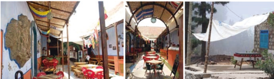
Fig. 3.35 Removable and adjustable shading: (1 and 2) the terrace of the Club Nautico in Mindelo (shading also using ships' sails), (3) shading of outdoor space of a house, using a single sheet
