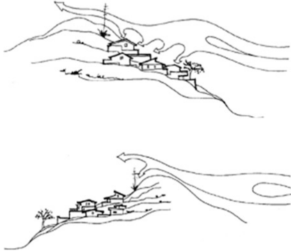
Fig. 3.12 On a hillside location, we must study the prevailing winds, in order to favour indoor ventilation
