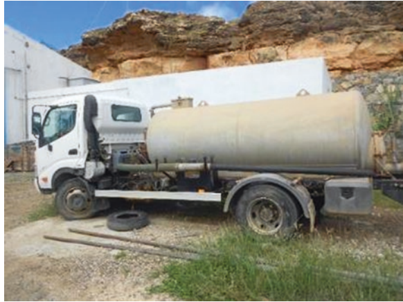
Fig. 16.18 Cleaning operation of a septic tank using a vacuum tank
