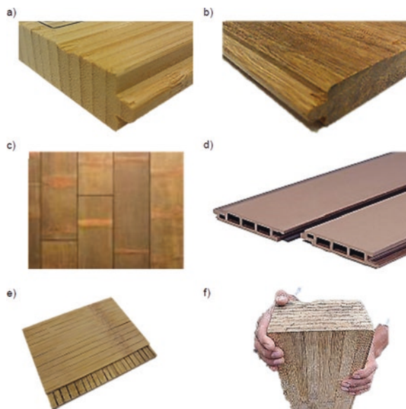
Fig. 15.4 Engineered bamboo products. Laminated bamboo: (a) ply bamboo and (c) flattened half bamboo poles (MOSO International B.V.) and (f) glue-laminated bamboo beams ( www.agenciadenoticias.unal.edu.co ). Densified bamboo: (b) SWB and other EBPs developed using Moso and bamboo, respectively: (d) bamboo plastic composite ( www.bambooindustry.com ), and (e) glue-laminated flattened bamboo boards
