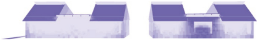
Fig. 7.15 Sunlight hours analysis. North facade during summer solstice, V1 (right) and V2 (left). Performance analysis: Dynamic simulation with EnergyPlus, Radiance, Daysim, and OpenFOAM in Grasshopper and Rhino
