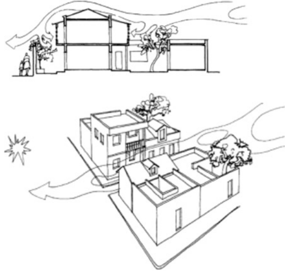
Fig. 3.16 The ventilation has a fundamental role, and one should focus on solutions to optimize the air circulation. The use of the courtyard-house typology is an effective measure in dryer climates such as in regions of Angola, Cape Verde and Mozambique. The issue of natural ventilation is further developed in Sect. 3.7, ahead
