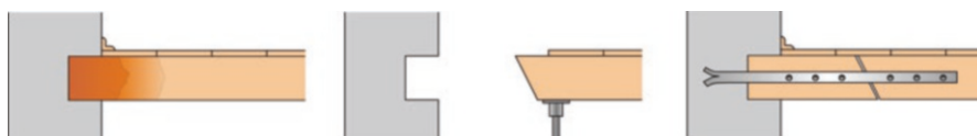
Fig. 14.14 Repair of a beam end using a timber prosthesis connected with metal plates and bolts
