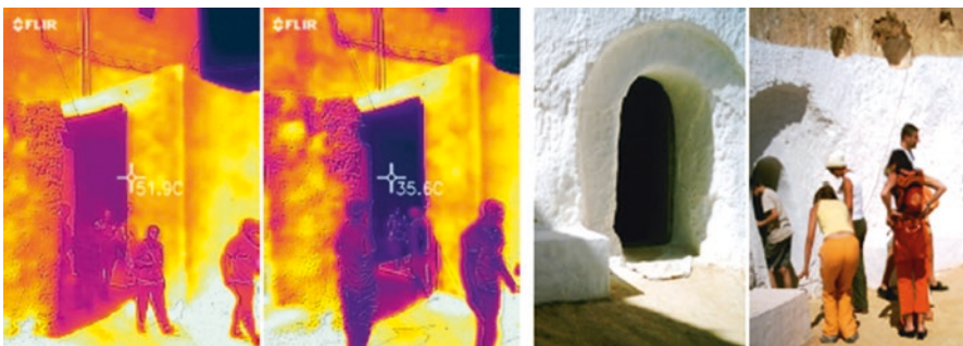
Figs. 3.114, 3.115, 3.116 and 3.117 Both on the left, thermal image comparison of the building thermal behaviour, showing the material interior surface temperature much lower than the measured temperature of the material external surface; both on the right, example of the Excavated Earth technique, showing entrance to a house built by extraction
