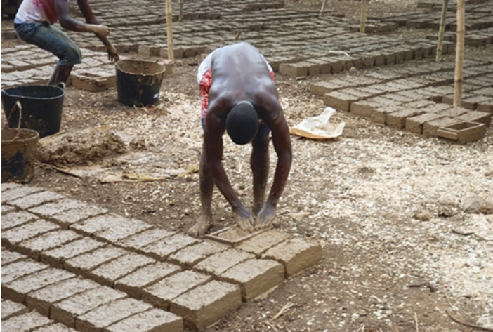
Fig. 13.1 The manufacture of adobe bricks in S. Tomé island
