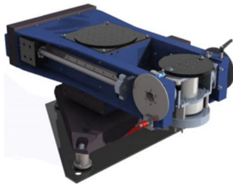
Fig. 10 Centrifuge with swinging rotor and drive counterweights
