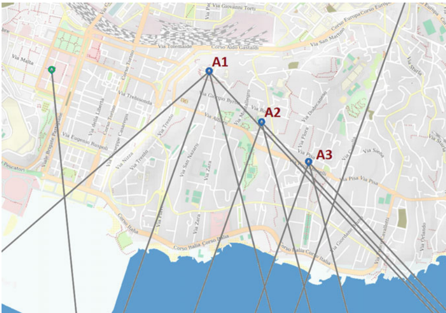
Fig. 4 Map of the experimental field site in Genoa (Italy) and horizontal projection of the microwave links. Sites A1 and A2 are equipped with tipping-bucket rain gauges (TBRG)
