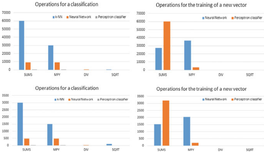
Fig. 1 Number of operations necessary for the 300 (above) and 15 (below) input vector size
