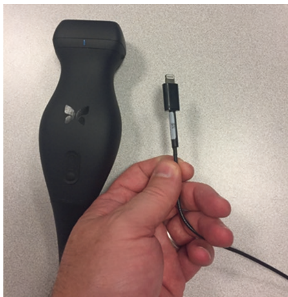
Fig. 16.3 Hand held, multimode, semiconductor chip ultrasound transducer connects to iOS mobile phone, uses cloud storage, and costs less than US$2000. Source: Jay Doucet (Author)
