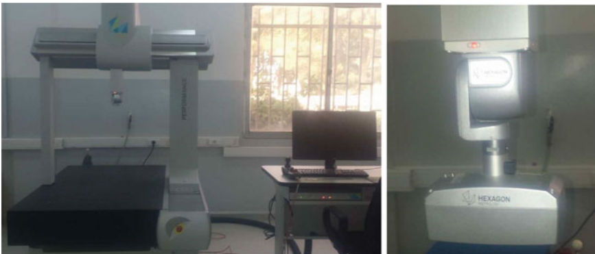
Fig. 2 Coordinate measuring machine and laser scanner
