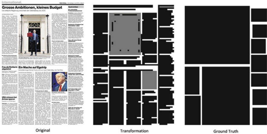
Fig. 12.6 Example of our dataset showing an original scan of a newspaper page (left), the transformed representation (middle), and the manually created segmentation mask (right)
