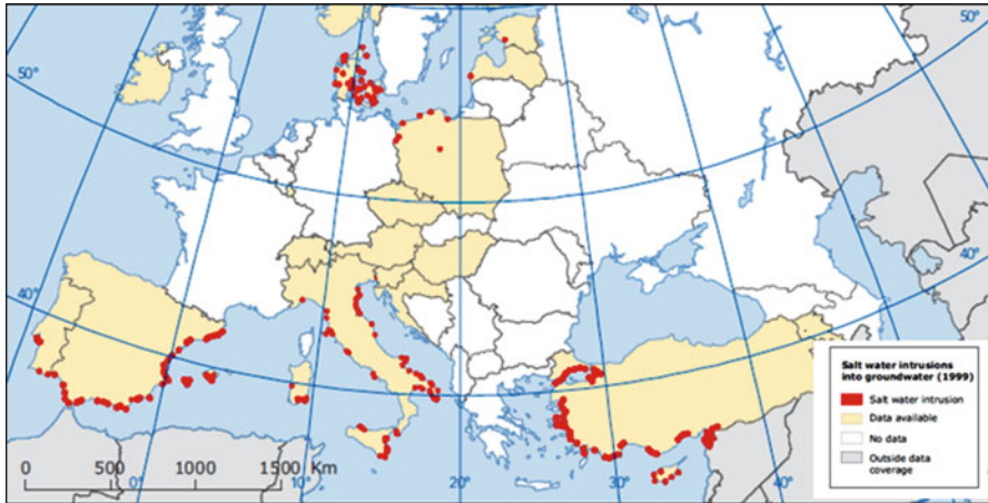
Fig. 7.4 Saline intrusion in Europe (EEA 2009)
