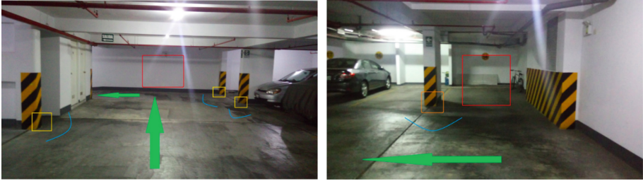
(a) Detection of objects, walls and signals of beacons. See the colors: yellow (beacons), red (object detection field), green (direction of route) and celestial (Bluetooth signal). (b) Positioning of the beacons in the parking lot. See the colors: yellow (beacons), red (object detection field), green (direction of route) and celestial (Bluetooth signal).
