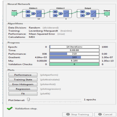
Fig. 6. Architecture of the neural network used for the prediction of CO_2 . It can be seen that the convergence occurred in the 14 th iteration, and there was no significant variation between the performance obtained in a previous iteration and the iteration immediately after.
