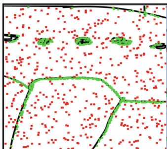
Fig. 4. Visualization of the results obtained using Spark feature. The green dots are the coordinates where a stroke was detected. (Color figure online)
