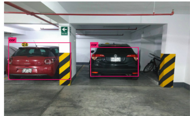
(b) Car detection in subway garage using tiny YOLO model.
