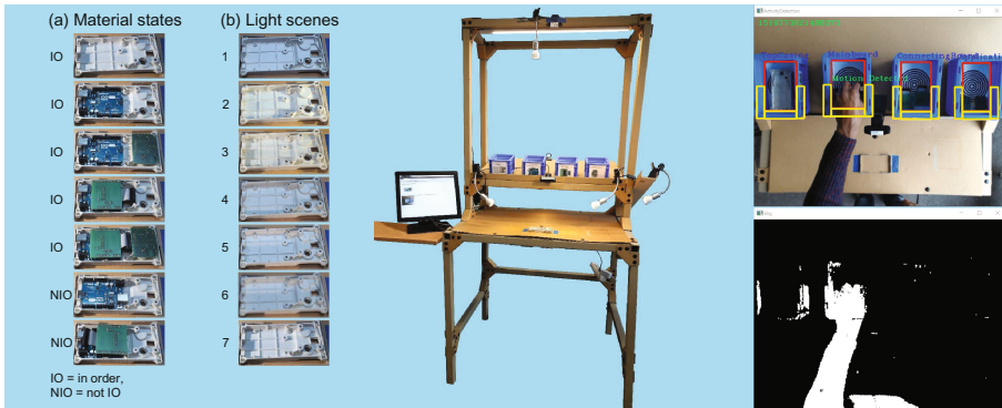
Fig. 2. Assembly workstation equipped with 1 touch screen, 2 cameras and 6 light sources (middle); example material states and 7 light scenes for one part (left); grasp detection using background subtraction with the ‘U’-shaped activity zones (right).
