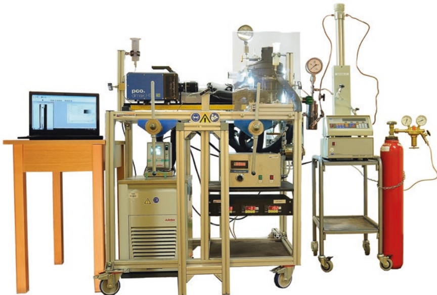
Fig. 5.2 Experimental high-pressure facility for the investigation of the oil droplet rise behavior in countercurrent flow with oil presaturation at Hamburg University of Technology. The shown setup corresponds to the flow diagram in Fig. 5.4 without the part inside the dashed box
