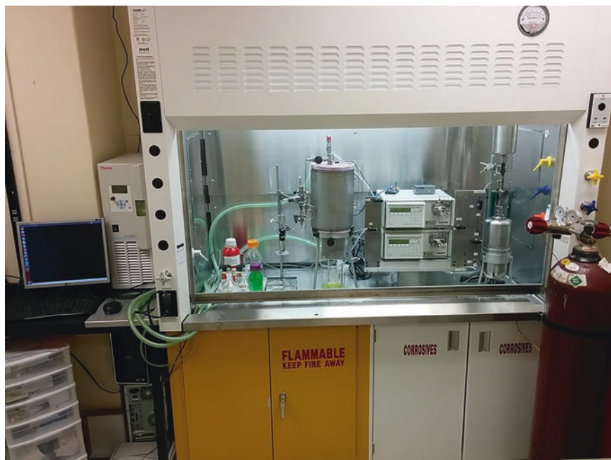
Fig. 8.2 Picture of the partition device showcasing the device, along with the computer controller for the thermometers and pumps, nitrogen and methane cylinders, and the recirculating water chiller
