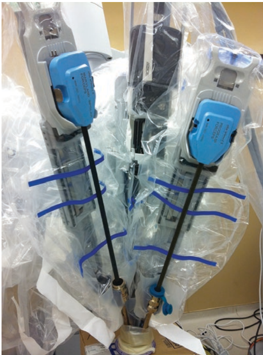
Fig. 16.2 With vertical docking of the Si platform and the QuadPort+, the first dry laboratory experiments were conducted for robotic TAMIS in September, 2010. Arrangement and working arm encroachment were among the parameters assessed in the first preclinical assessment of robotic TAMIS
