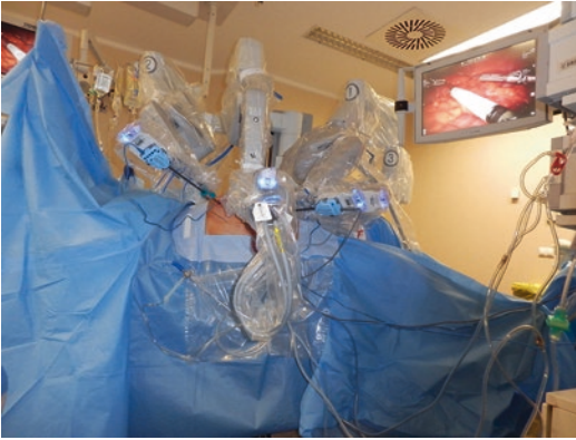
Fig. 44.1 Da Vinci Si System docked from the left lateral side of the patient
