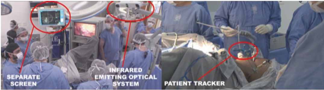
Fig. 47.1 A stereoscopic infrared emitting optical system continuously tracks the patient and instrument by detecting infrared light which is reflected by marker spheres affixed to a patient tracker and an instrument tracker. On
