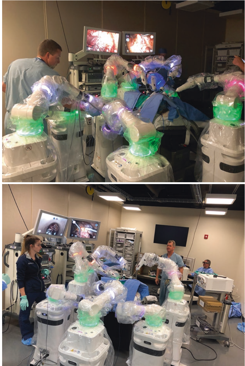
Fig. 45.5 The CMR modular versus platform allows surgeons to operate in two fields simultaneously to perform two-team taTME. (Photo courtesy of Sam Atallah, MD)
