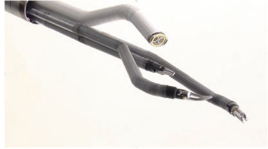
Fig. 17.3 The da Vinci SP system's single 25-mm cannula through which three 6 mm, multi-jointed, wristed instruments and a 3D 0° HD camera extend
