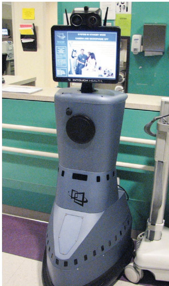
Fig. 17.1 RP-7 Robot (InTouch Health Santa Barbara, CA). Self-propelled robot with bidirectional audiovisual communication is one method of engaging with patients in tele-ICUs
