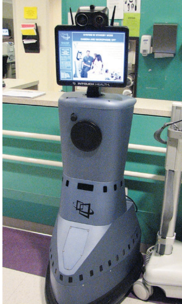
Fig. 17.1 RP-7 Robot (InTouch Health Santa Barbara, CA). Self-propelled robot with bidirectional audiovisual communication is one method of engaging with patients in tele-ICUs
