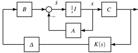
**Fig. 4** Small-gain setup of systems with time-varying delay
