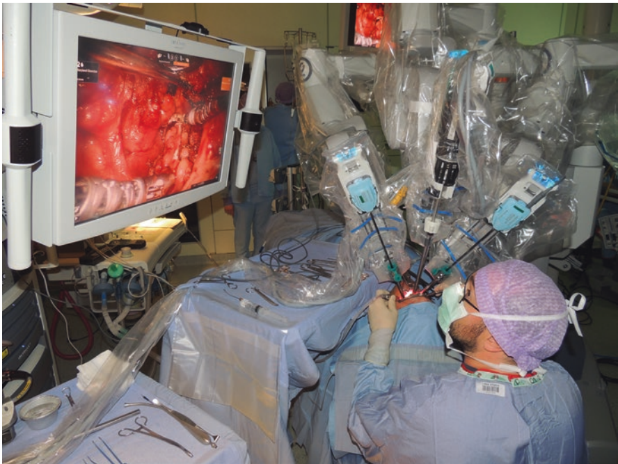
Fig. 6.1 Operating room during TORS. The bedside assistant can follow all the surgical steps on the monitor while the first surgeon is working at the robotic console
