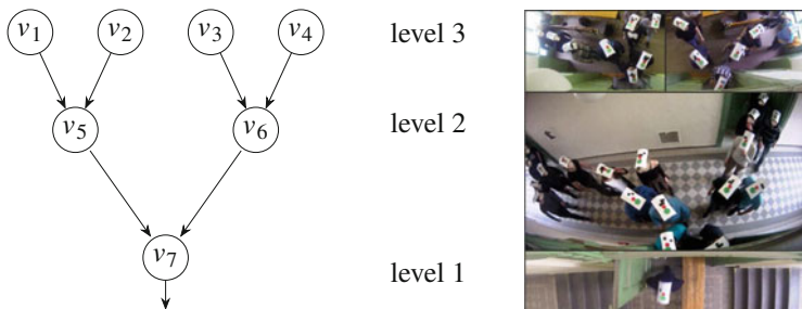
Fig. 1 Schematic illustration of the experimental layout. Students were leaving the lecture room via a tree-like structure of consecutive bottlenecks. The experiment was recorded by four cameras placed above the exits v_5 to v_7
