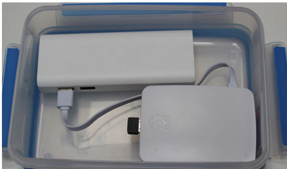
Fig. 2 This figure shows hardware in a waterproof box. The setup comprises a power bank, a USB-power-connector, a WiFi -dongle, a microSD -card, and a Raspberry Pi
