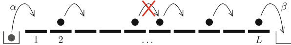
Fig. 1 The TASEP consists of L cells, which are either empty or occupied by maximally one particle. If a site is chosen to be updated and is occupied by a particle, the particle can jump to the next site, if the next site is empty. The case of open boundary conditions is shown, where site 1 feeds from a reservoir which is occupied with probability \alpha and site L exits into a reservoir which is empty with probability \beta
