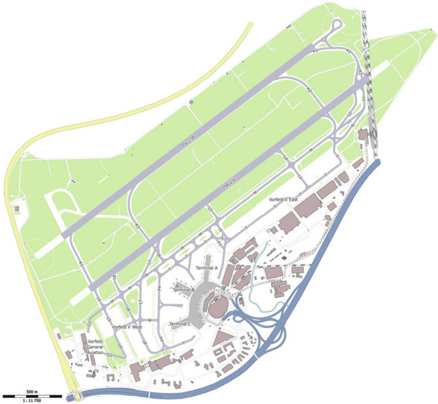
Fig. 1 Layout of Duesseldorf Airport (EDDL). The airport consists of two parallel runways (05R/23L and 05L/23R) and one main taxiway (M). Furthermore there is one passenger terminal with terminal parts A, B, and C and a main apron, the apron west, and the apron east. Source: OpenStreetMap contributors (Licence ODbL) [11]
