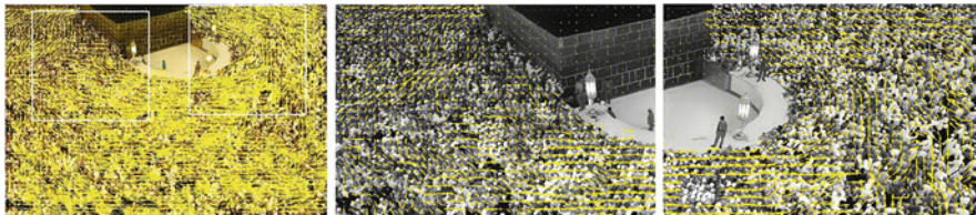
Fig. 1 Input image and vectors of first dataset. Magnified views accurately show the direction of crowd movement
