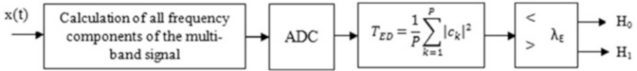
Fig. 11.1 Block diagram of a frequency domain energy detector based on the c_k frequency components for the band of interest
