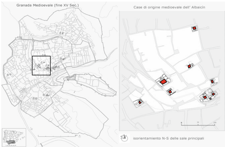
Fig. 5 Orientation N-S and internal patios (red color) of the main mansions in XVI Century Granada
