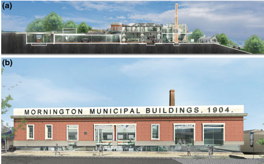
Fig. 9 a Final design showing north-south sectional perspective/underpass. b Final design showing raised 1903 part of the Mornington Cable-Car Depot building above the original 1882 basement, with gap between. Renderings by Author
