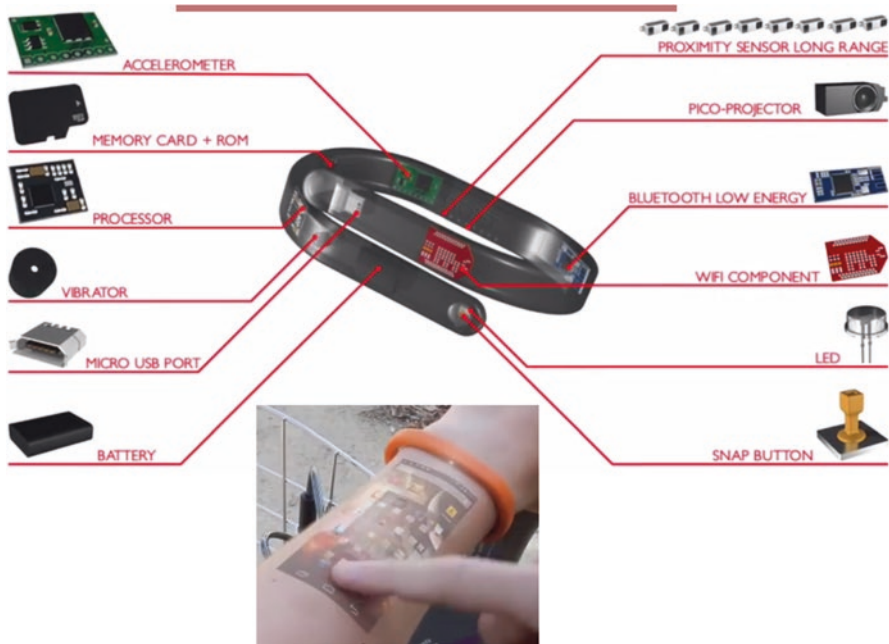
Fig. 3.13 Circlert Bracelet and the integral components. The inset shows working of the Circlert Bracelet on the arm of the user. Reproduced with permission from Circlert
