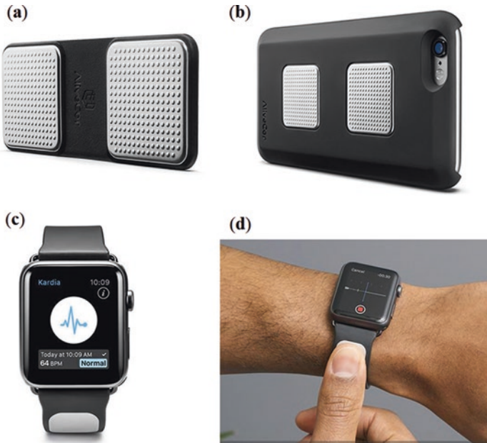
Fig. 3.4 SPMHDS developed by AliveCor, Inc. (a) Kardia Mobile. (b) Kardia Mobile in iPhone 6 cover accessory. (c) Kardia Band. (d) Kardia Band's operational procedure. Reproduced with permission from AliveCor, Inc. Images provided are courtesy of AliveCor, Inc.
