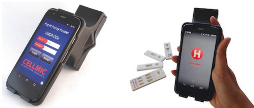
Fig. 1.1 A holomic rapid diagnostic reader (HRDR) for the readout of lateral flow immunoassays. Left: HRDR-200. Right: HRDR-300. Reproduced with permission from Cellmic, USA
