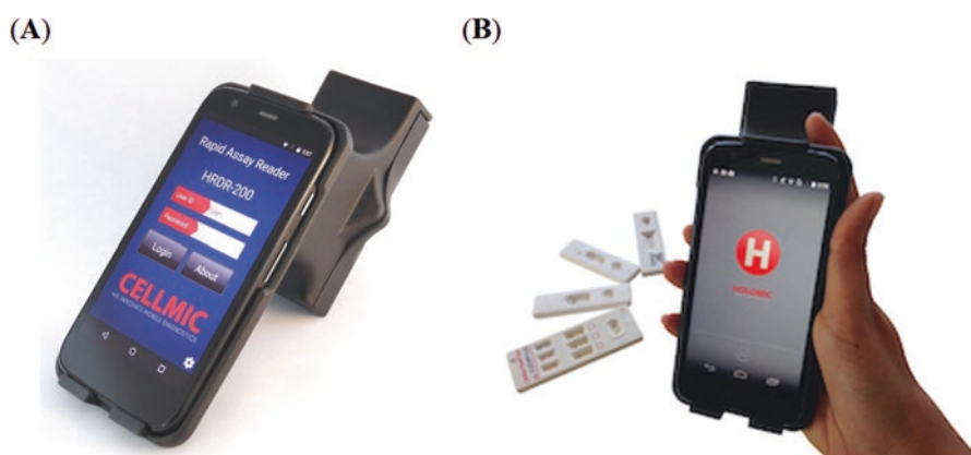
Fig. 5.9 Smartphone-based readers for rapid diagnostic tests developed by Cellmic. (a) Holomic Rapid Diagnostic Test Reader (HRDR-200) (b) HRDR-300. Reproduced with permission from Cellmic
