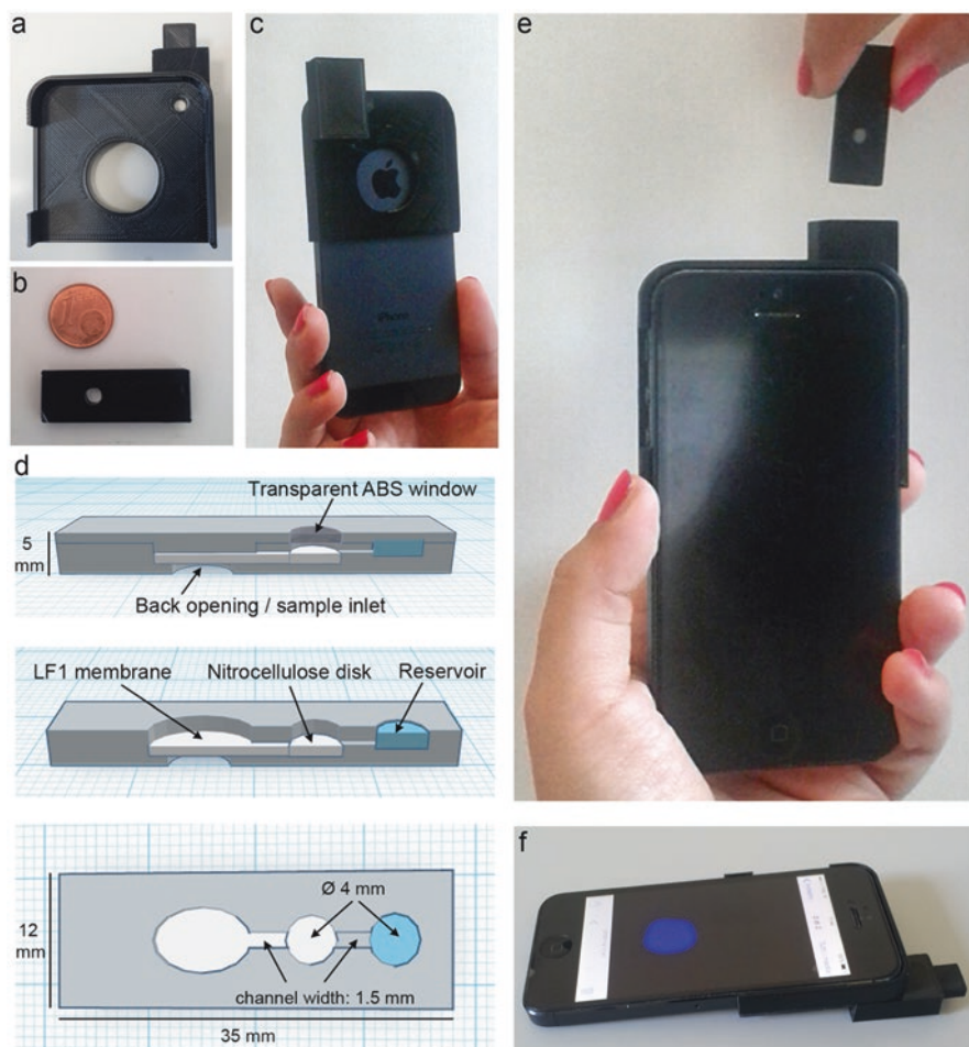
Fig. 2.11 An SP-based device for the detection of luminescence [127]. (a) SP attachment. (b) Mini-cartridge. (c) The SP attachment snapped into the SP. (d) Schematic of the mini-cartridge showing the various components, where the transparent ABS window (200 \mu\text{m} thick, 4 mm diameter) allows the imaging of luminescent reaction by the SP back camera. (e) Insertion of mini-cartridge into the SP attachment. (f) Luminescence signal acquisition by the SP. Reproduced with permission from the American Chemical Society
