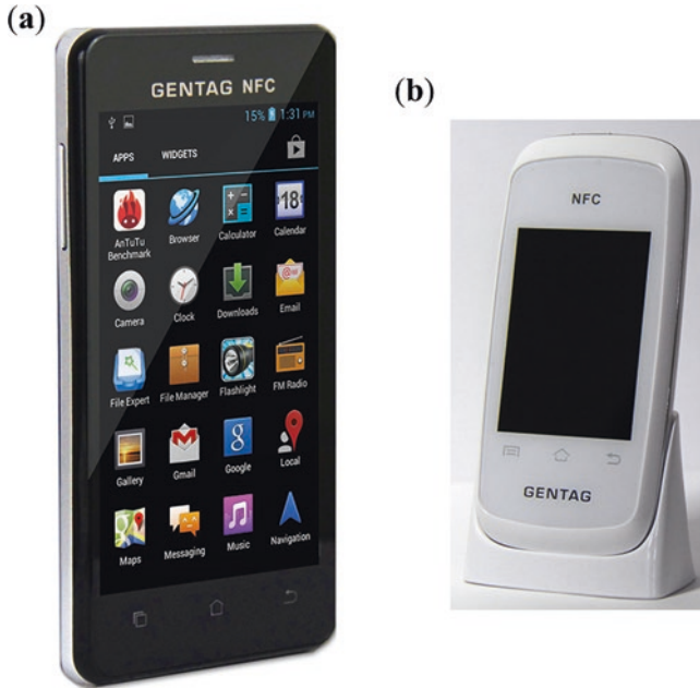
Fig. 3.5 SPMHDs by GENTAG, Inc. (a) NFC Smart Cell Phone and (b) NFC Sensorlinker. Images provided by Dr. John P. Peeters, GENTAG, Inc. Reproduced with permission from MDPI [92]
