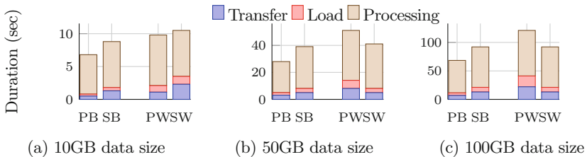
Fig. 5. Effect of tuning homogeneous data sizes with 10 GB, 50 GB, and 100 GB heterogeneous input data size. PB stands for BigDAWG performance with tuned data distribution, SB stands for Spark performance with tuned data distribution (the same distribution as PB), PW stands for the worst BigDAWG performance, and SW means Spark performance with homogeneous input data same distribution as PW.
