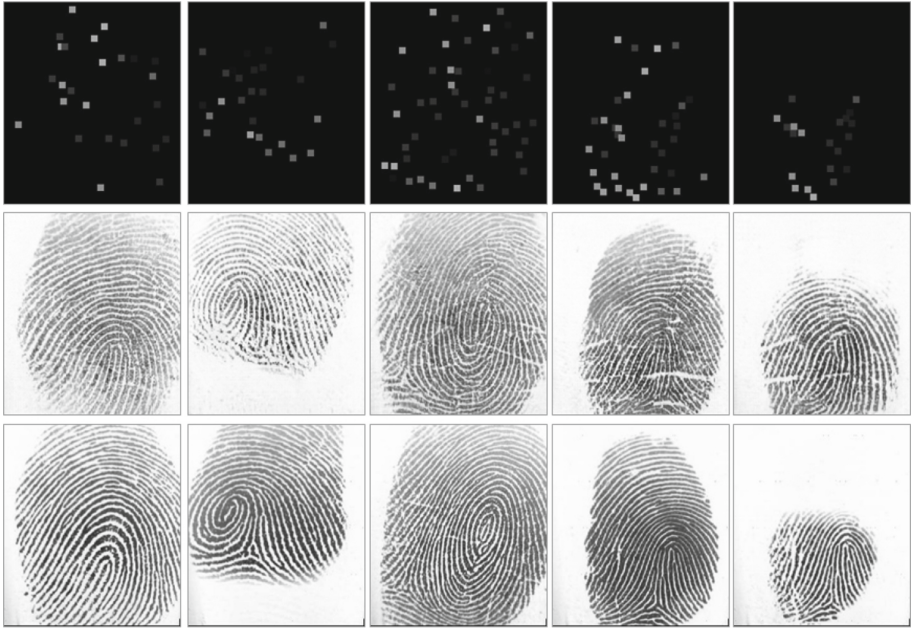
Fig. 5. Samples of reconstructed fingerprints. First rows: minutiae maps; second row: fingerprints generated from the minutiae maps by the proposed network; third row: real fingerprints from which the minutiae were extracted.
