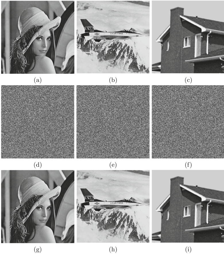
Fig. 4. Test images applied on the proposed algorithm. (a)–(c) are the original images of Lena, Airplane and House respectively; (d)–(f) are the marked-encrypted images of Lena, Airplane and House with the total embedding capacity when embedding in three bit planes respectively; (g)–(i) is decrypted images of Lena, Airplane and House respectively.
