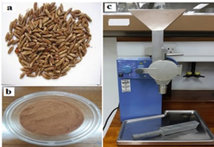
Fig. 6.4 Waste date pits (a) original form, (b) powder of waste date pits and (c) grinder used for grinding
