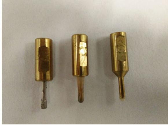
Fig. 14.3 ASAP-1 tools. From left to right: Diamond tool, Xylem tool, and Xybove tool
