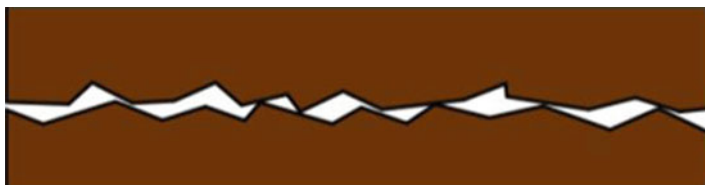
Fig. 7.11 Contact resistance at a mechanical joint is due to the surface roughness on a nano scale. The gaps need to be filled either by a filler material such as indium or the contact force has to be very high
