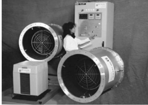
Fig. 1.21 Cryopump for a space simulation chamber [139]
