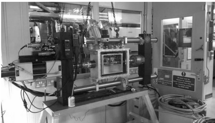
Fig. 4.4 Experimental set-up for the measurement of internal stress in engineering materials under loads. The uniaxial load up to 100 kN is provided by hydraulic loading rigs
