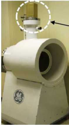
Fig. 9.6 GE 0.5 T conduction-cooled head imaging system [6]
