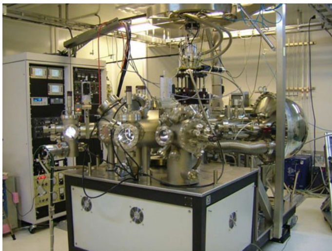
Fig. 7.26 A cryocooler mounted on a UHV vacuum chamber for surface analysis. (Courtesy Prevac, Poland)
