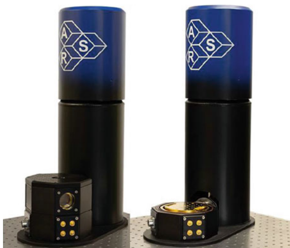
Fig. 7.14 X23 cryostat for nano-optics. The cryostat design is for a high numerical aperture for near-field experiments. In the figure on the left, the objective is seen inside the vacuum space to minimize the distance from the sample to the objective. The sample plate is supported on an ultra-low expansion support to minimize any drift during temperature ramping of the sample. ARS drawing
