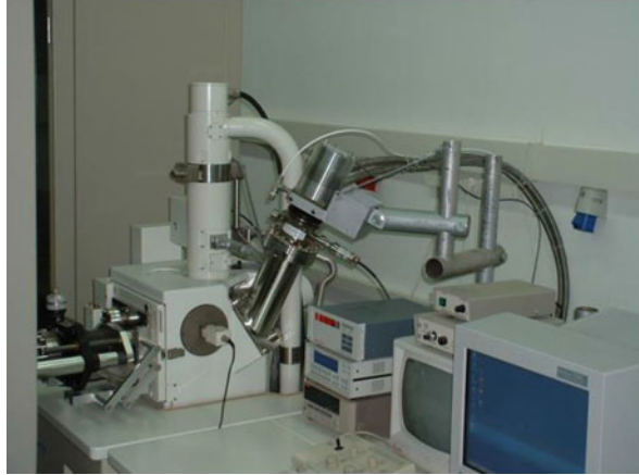
Fig. 7.27 ULV cryostat use on an SEM microscope. (Courtesy Prof. Dan Rich, Ben Gurion University, Israel)
