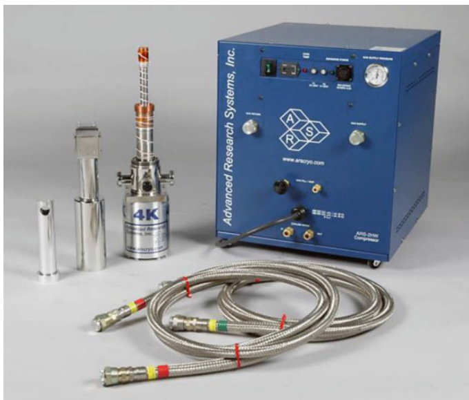
Fig. 7.3 Components of a typical cryostat. From top left, clockwise, radiation shield, experimental vacuum shroud, cryocooler, helium compressor and helium hoses (to connect the cryocooler to the compressor). ARS picture gallery
