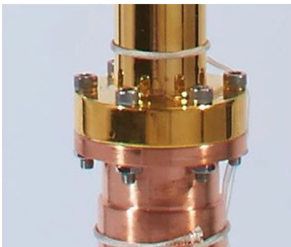
Fig. 7.11 Contact resistance at a mechanical joint is due to the surface roughness on a nano scale. The gaps need to be filled either by a filler material such as indium or the contact force has to be very high
