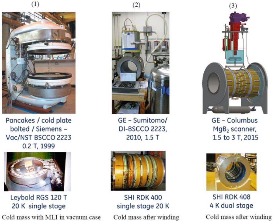
Fig. 9.5 Cryocooler integration—small-scale HTS MRI
