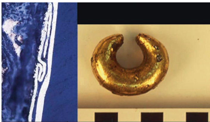
Fig. 6.9 Foil-gilded penannular nose ornament from the site of La Compania, Los Rios Province, Ecuador, from the tenth century AD secondary chimney urn burial. The section through part of the surface shows corroded copper beneath a typical gold foil covering where folds can be seen in the foil. Unetched, magnification on left is x75. Scale bar on the right is in centimetres
