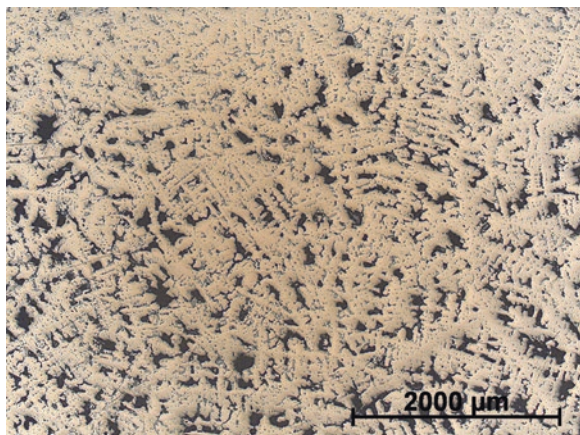
Fig. 4.21 Heavy cored bronze casting waste from the oppidum of Manching, Germany with dendritic appearance of pores. Unetched specimen containing 9.5% tin and 7.2% lead
