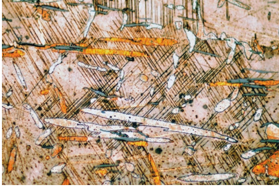
Fig. 4.45 Thai bronze bowl from the site of Ban Don Ta Phet, showing twinned alpha grains in a beta matrix. These twinned grains arise from the casting, heat treatment, quenching from about 650 °C, then reheating, hot-working, and subsequent quenching of the 22.7% tin bronze alloy, resulting in a beta or beta and gamma phase matrix with twinned alpha phase islands. Colour etched in Klemm's reagent II, magnification 280×
