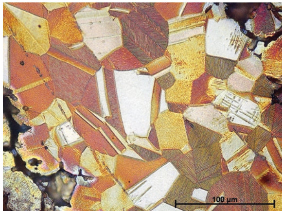
Fig. 3.12 Recrystallized \alpha -brass of a gladiator helmet from Herculaneum (see also Figs. 3.21 and 5.17). Klemm's reagent II has produced pattern of parallel lines on the individual twins and grains which are related to their crystallographic orientations
