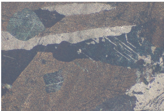
Fig. 5.38 Section across a tin ingot, showing columnar grain growth. Chill cast, 99.9% tin
