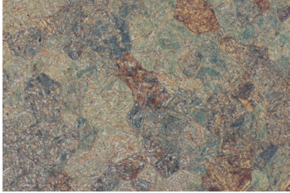
Fig. 5.19 A 60% copper and 40% zinc cast laboratory ingot showing the alpha + beta structure of these high-zinc cast alloys. The microstructure consisted of beta grains at high temperature, which then break down into grains of alpha + beta, outlined by the former beta grain boundaries. Colour etched, magnification \times 180
