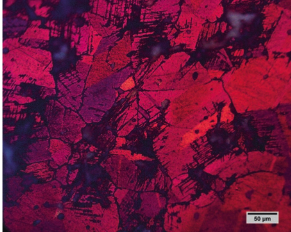
Fig. 4.36 Cold-worked cutting edge from a Late Bronze Age palstave from Kent with about 8.5% tin. Corrosion has outlined the strain lines through the grains seen here. Lightly etched in alcoholic ferric chloride
