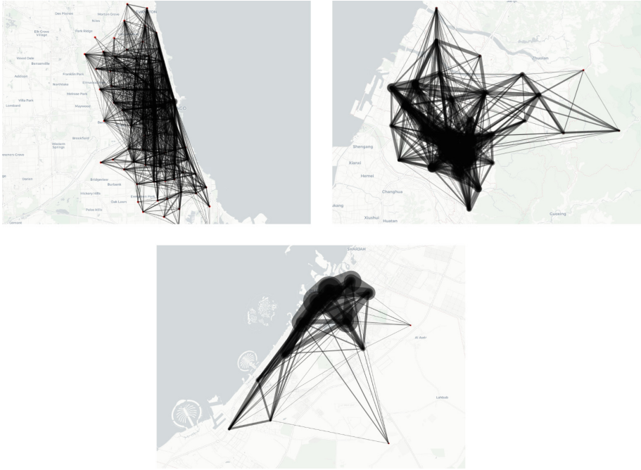
Fig. 3. The Graph G_2 for the cities of Chicago (top-left), Taichung (top-right) and Dubai (bottom). Line thickness is related to number of lines attending two nodes.
