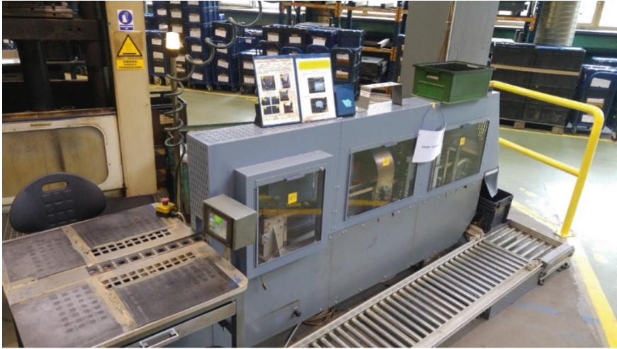
Fig. 6. Machine to 100% control of adhesion of car steering column couplers.
